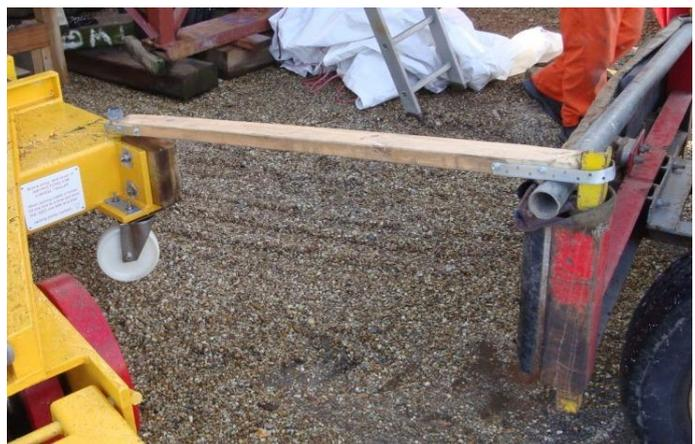
**Using the steel guide arms** (NB. only one trailer has sockets for the arms.)
